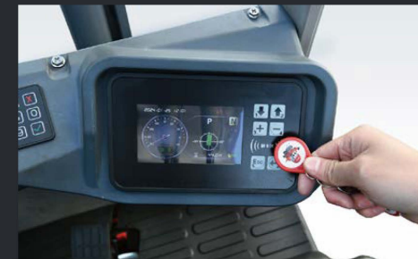
The integrated card swiping function of the instrument meets the requirements of TSG 81.
