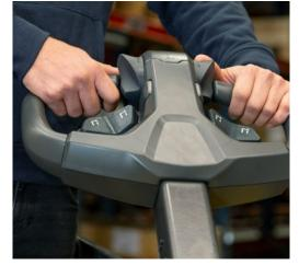
The class-leading, user-friendly *emPower* tiller head gives easy access to controls and enables rapid, precise operation.
